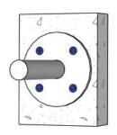
1. Back arm with round plate is secured to the wall using concrete screws to support the awning frame.
