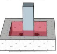
2. Footer hole that has a base plate welded to the bottom of a column and is then bolted to the footer. The hole is then filled with mortar to give a smooth surface.
