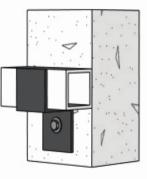
1. Z-Bracket is bolted to the wall and allows the square tube of the awning frame to be supported this option is for when mounting locations are limited due to places to secure the frame. Or if mounting points have not been determined on site.
