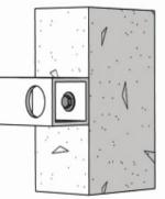
4. A Recess hole is cut into the square tube and the anchor bolt is then secured to the wall. This option is used for helping to conceal the anchor bolt from open view.
