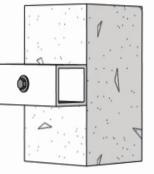
3. The Anchor Bolt is secured directly through the top of the tube and anchored into the wall. This is used when mounting points have not been determined.
