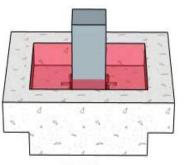
3. Footer hole that has Rebar welded to the column to add stability and is then filled with mortar to give a smooth surface. The rebar also acts as a floor support.
