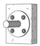
2. Back arm with round plate is secured to the wall using anchor bolts to support the awning frame.
