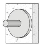
3. Back arm with a round plate that is secured to the wall using either concrete screws or anchor bolts. It is concealed with a cover plate to give a cleaner appearance of the wall mounting.
