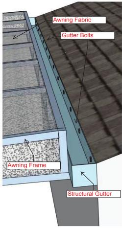
With a Structural Gutter you are able to secure to the wall of the building its heavy gauge materials allow it to become an option for supporting the weight of an awning frame. The Gutter is directly bolted to the wall and acts not only as a water diversion but also as support for the frame. The Awning is usually bolted directly to the gutter itself. As a different approach arms can be extended up under the gutter and secured directly to the wall as well to support the awning.
