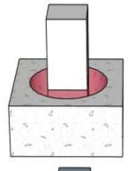
1. Core drilled into the concrete slab that allows for the awning column to be placed in and then fill the hole with mortar to give a smooth surface.
