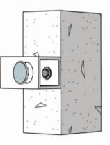
5. A Recess hole is cut into the square tube and the anchor bolt is then secured within the tube to the wall Button Cap it is then covered with a Button Cap to help conceal the location of the Anchor and provide a cleaner appearance.
