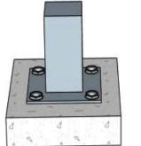
4. The column has a base plate welded to it and is then bolted directly to the concrete slab.
