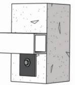
2. Square Tabs are welded to the square tube of the awning frame and bolts are used to secure it to a wall. This option is ideal for when mounting points have been determined prior to site arrival
