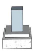
5. The column has a base plate welded to it and is then bolted directly to the concrete slab. There is a cover plate used to conceal the bolts to provide a cleaner look and reduce a possible trip hazard.
